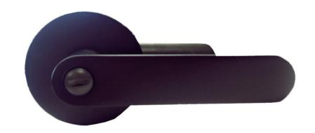
Heavy Duty tubular ENTRANCE & PRIVACY Function lever handle on round rose,60/70mm adjustable backset, stainless steel face plate in oil rubbed bronze finish, fit for door thickness 40-50mm
